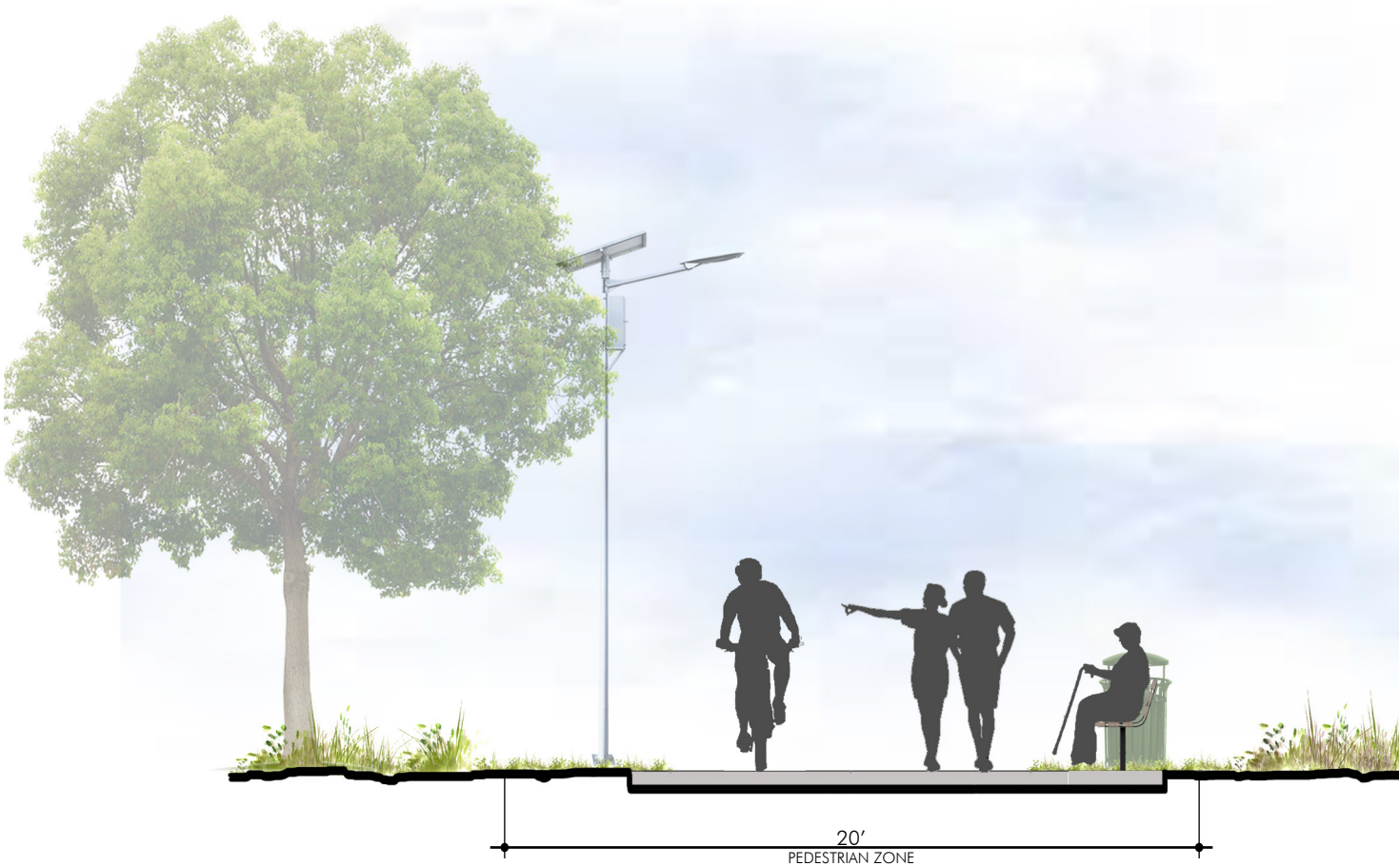
Prototypical trail section with ideal 20’ wide pedestrian zone. Amenities may consist of 6’ bike lane, 6’ pedestrian lane, seating, lighting and buffer zones
